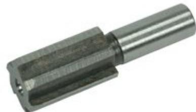
Wildcat conversions using the .224" bullet with .2200" inside neck diameter and .243" bullet with .2390" inside neck diameter, Forster offers inside neck reamers for these sizes. Use after the CASE sizing operation.
