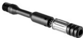
\* Vepr and Saiga Pistons will require drilling through the op-rod after screwing the piston into the carrier, due to variations in the staking location. These Op-Rods are Phosphated instead of Nitrided to allow easy drilling.\*
