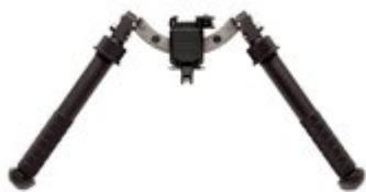
Mounts directly to any 1913 style Picatinny rail via included CUSTOM ADM Lever. Height Range approximately 5.5 - 10.5" 15 degrees +/- of preloaded Pan. 15 degrees +/- of preloaded Cant. 5-H Pan and Cant can be locked out at top dead center PAN and CANT Tension Wheel has Detent adjustability and Cam-Lock PATENTED multiple deployable leg positions of 0, 45, 90, 135 and 180 Non-Rotating Legs\* Weight 26 ounces. Available in black only
