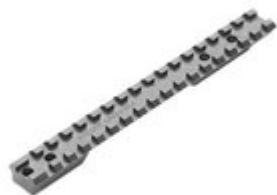
Heavy steel base with 20 M.O.A. forward angle increases maximum scope elevation for long range shooting. Machined after hardening to maintain dimensions. Integral recoil lug withstands the hardest kicking calibers. Uses MIL-STD 1913 Picatinny slot pattern for maximum sight mounting possibilities. Remington Zero Cant does not have 20 M.O.A. forward angle. For use where extra elevation is not required. Fits 700 short action only.
